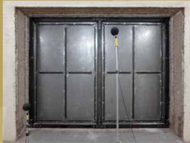
A large scale, 3600x2800mm RW 55dB RHINO-HM TVF room door on test at the University of Salford Acoustic Test Laboratory to BS EN ISO 10140-2
